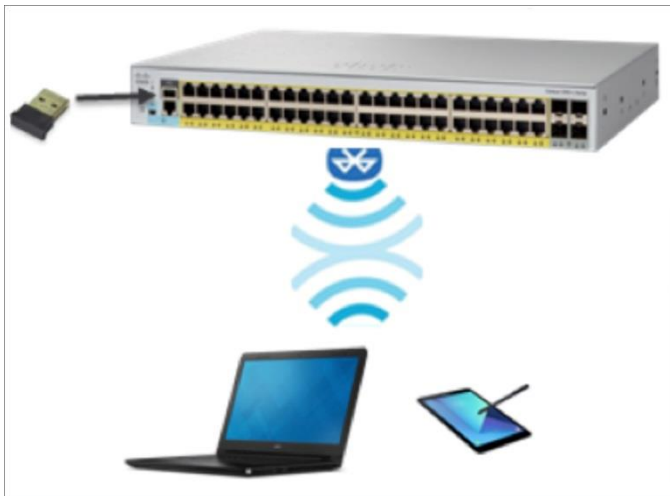
Figure 2. Over-the-air switch access using Bluetooth
